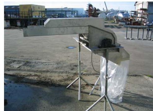
Fig 4 – Hogger prior to installation on Sureste 709
