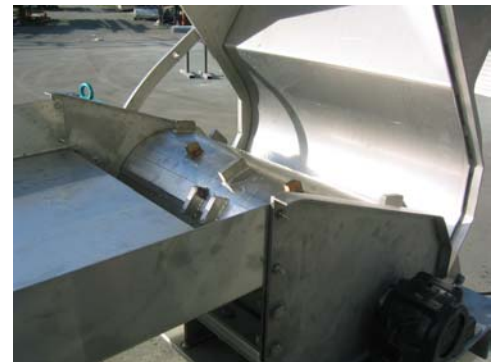
Fig 3 - Internal details of Hogger showing teeth and upper lid assembly
